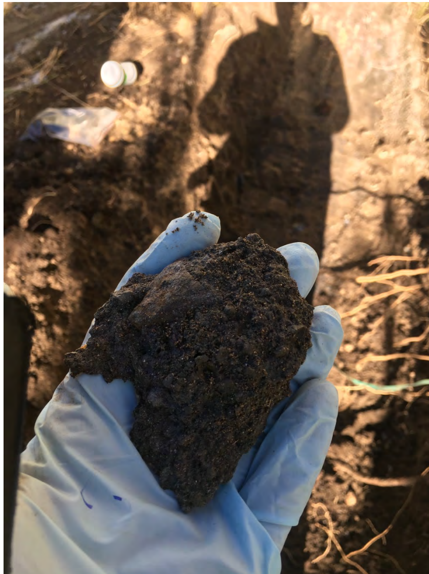
Photo 16: Latite and clay material sampled from test pit TP103 (24 July 2019)
